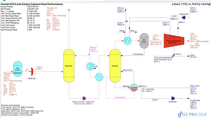
CO<sub>2</sub> Capture System of a typical SIEMENS ENERGY 1-1-1 SGT-5 9000HL Gas Turbine Combined Cycle Plant
